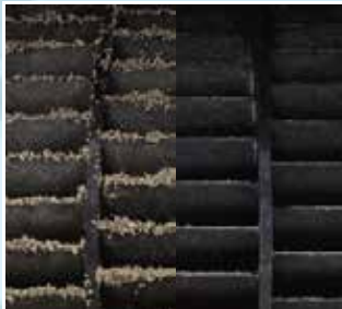
Image after 10 years | Dual Barrier Coating used
